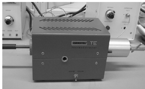
Figures 3.1-2a and b. (a) Scheme and (b) photograph of the Thermal Extractor TE2 [Scheme according to: Scherer et al., 2006b].
